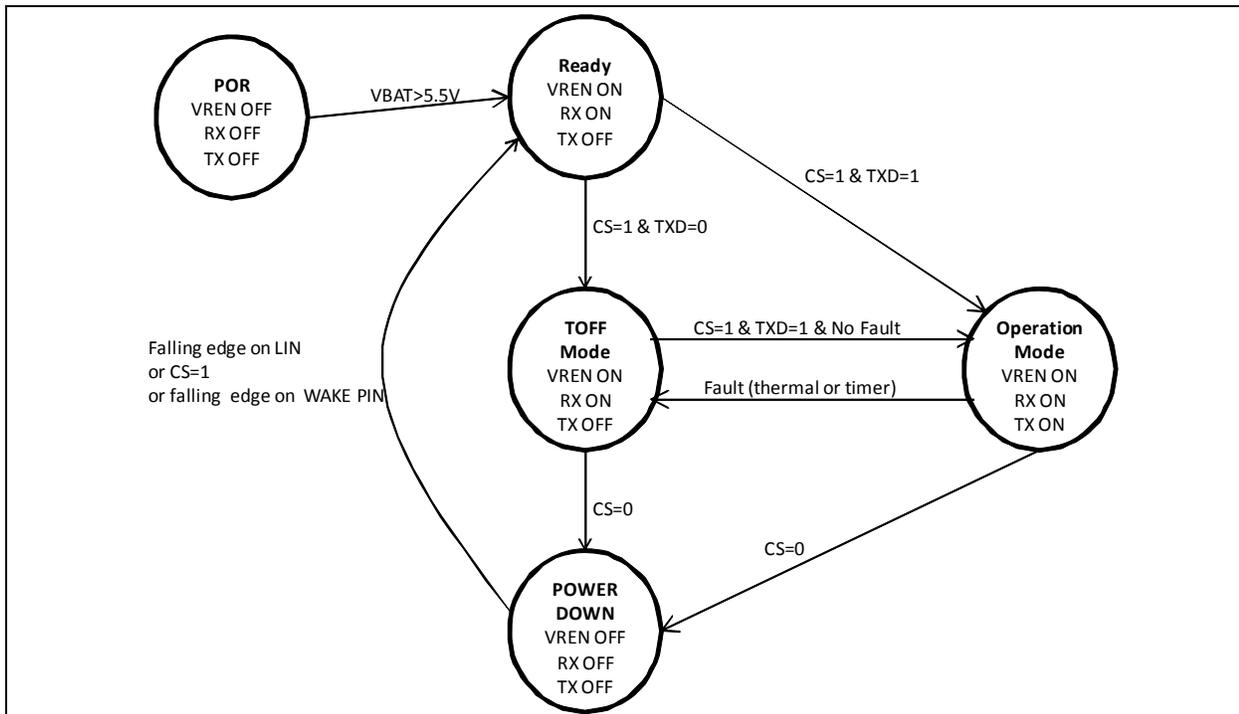
**FIGURE 1-3: OPERATIONAL MODES STATE DIAGRAM – MCP2003A**
