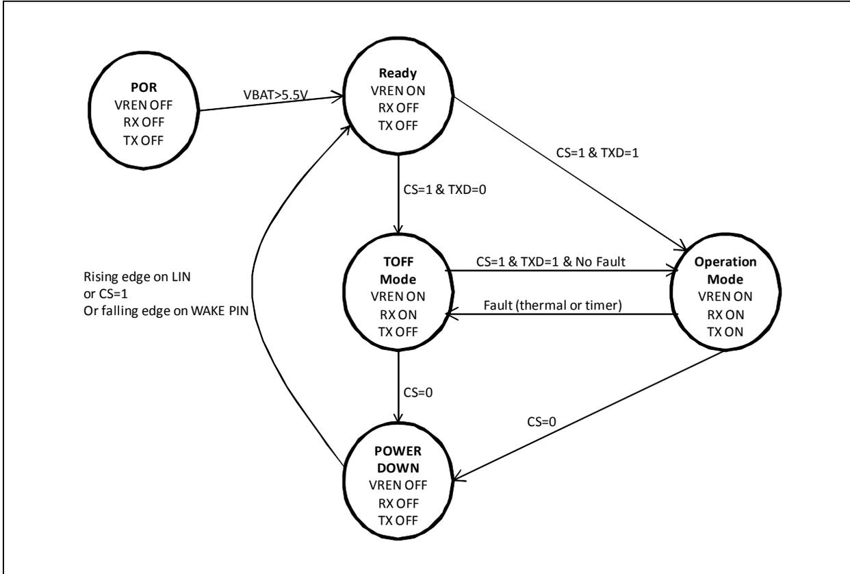
**FIGURE 1-4: OPERATIONAL MODES STATE DIAGRAM – MCP2004**
