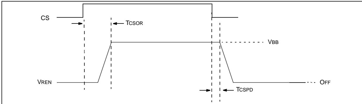
**FIGURE 2-6: MCP2003/4 REMOTE WAKE-UP**
